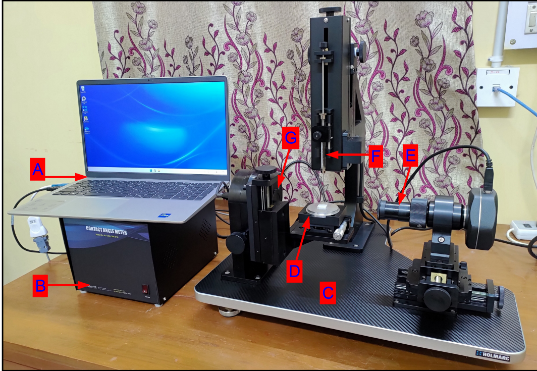
Figure 3.2: Digital image of the experimental setup: (A) Laptop for controlling the imaging and dispensing system; (B) drop dispenser controller; (C) rigid workbench for stable mounting of components; (D) substrate holder; (E) high-resolution camera; (F) micro-syringe; (G) LED light source with diffuser for uniform back-lighting.
