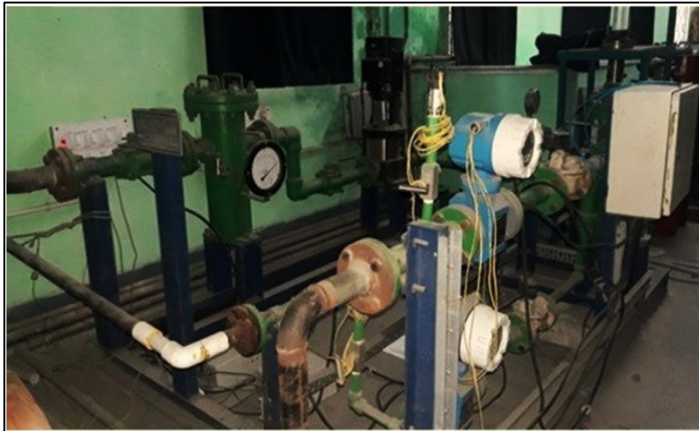
Fig. 3.1.9 Water Flow Circuit
