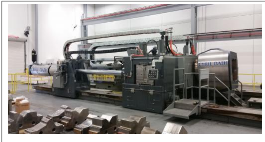
Figure 3.8 Photograph of Stretch Straightening Machine, Make: M/s. Cyril Bath Co., North Carolina, USA [78].
