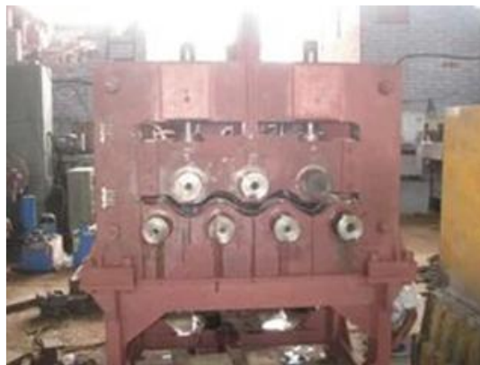
Figure 3.14 Photograph of Cluster Roll Straightening Machine [85]
