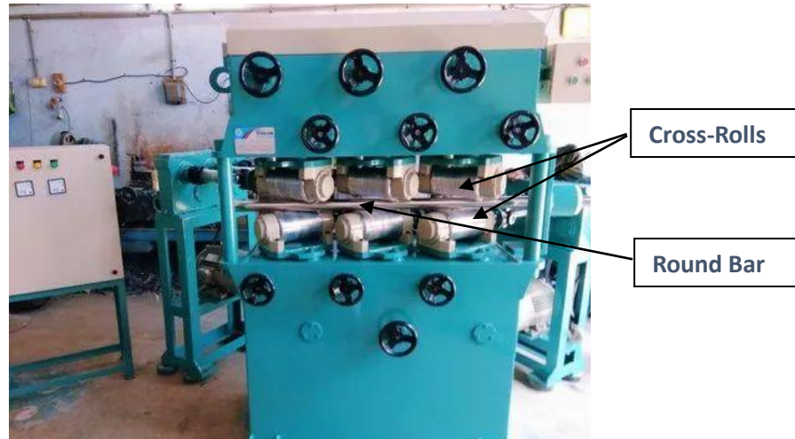
Figure 3.12 Photograph of Six Roll Straightening Machine. Brand: Shivam Engineering [83]
