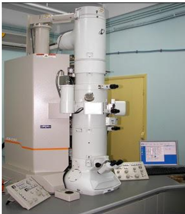
Figure 3.12: Experimental set up of HRTEM (JEOL JEM-2100)
