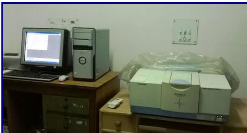
Figure 3.6: Experimental set up of FTIR spectrometer
