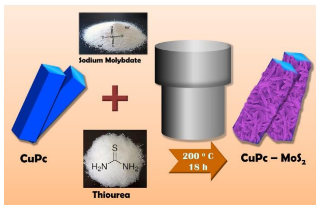
Figure 4.5: Preparation scheme of MoS 2 -CuPc heterostructure
