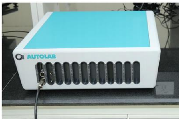
Figure 3.19: Set up of electrochemical workstation (Autolab PGSTAT M-204)
