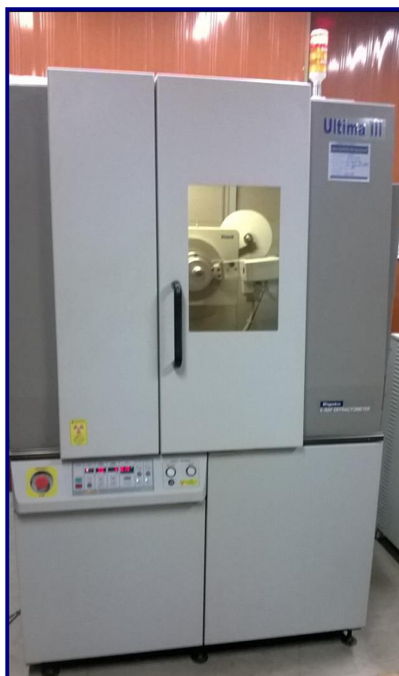
Figure 3.4: Experimental set up of X-Ray Diffractometer
