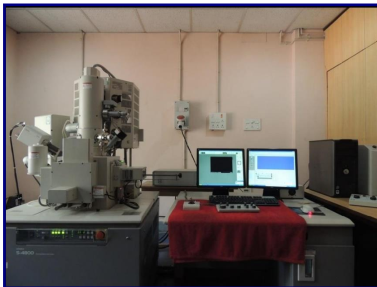
Figure 3.10: FESEM (Hitachi S-4800) set up with EDS attachment
