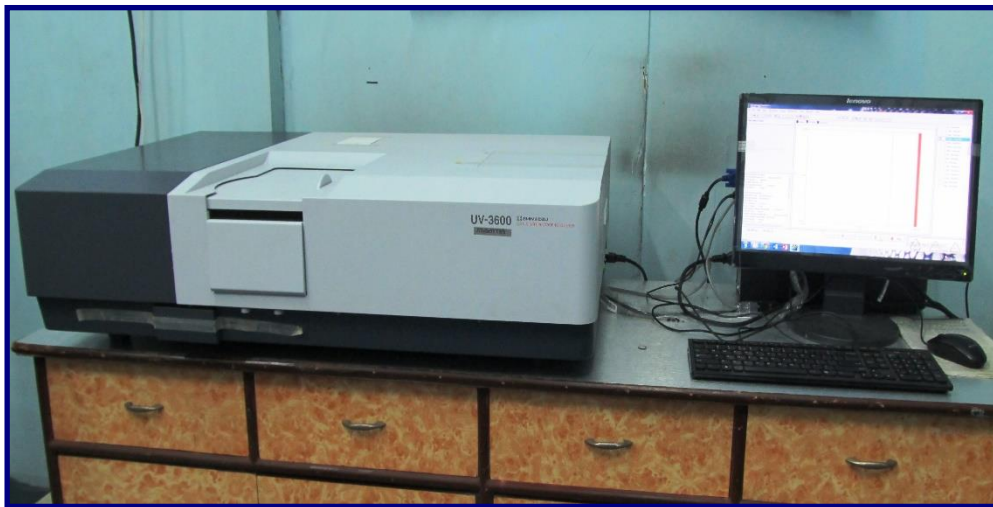
Figure 3.8: Experimental set up of UV-Vis spectrophotometer
