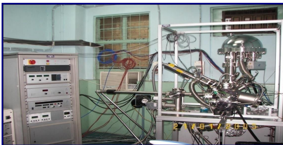
Figure 3.14: Experimental set up of XPS (SPECS HSA 3500)
