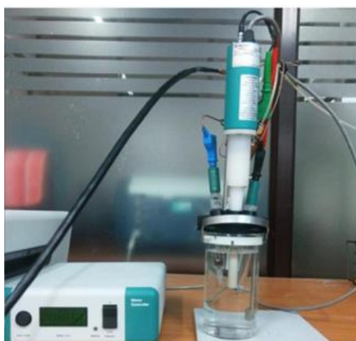
Figure 3.20: RDE measurement set up
