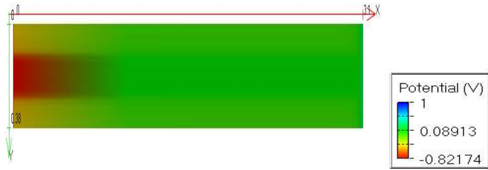
Figure 3.2: Electrostatic potential profile from the cathode to anode under an applied anode voltage of 0.55 V
